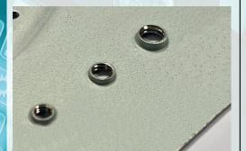
The ability to create M3 & M4 taps whilst we are processing at the blanking stage of manufacturing enables the ability to create tapped holes via an automated process instead of adding a clinch nut at a later manufacturing stage using a separate machine and additional labour. The manufacturing efficiencies this provides ultimately provides additional savings when creating the end product.
